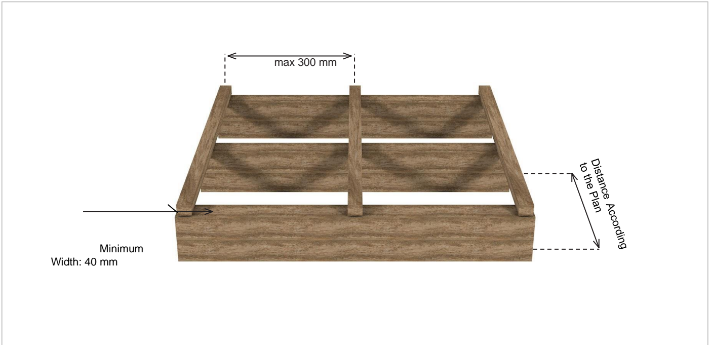
Figure 2: Joists on a Wooden Structure
